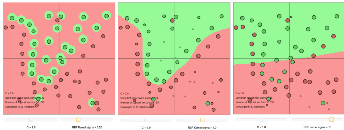
Figure 1.5: Using a too small (left), a nicely chosen (middle) and too large (right) radial basis function parameter \sigma .
